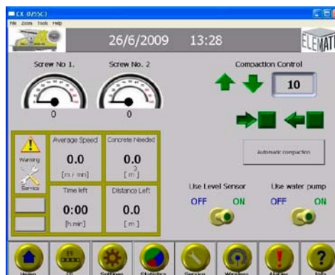
The touch-screen interface enables efficient production control and utilization of history data. Its three access levels prevent uncontrolled entries.
