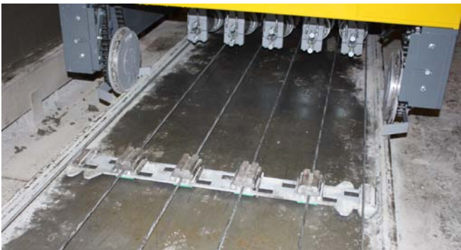
The advanced strand guide helps to meet the stringent strand location tolerances.
