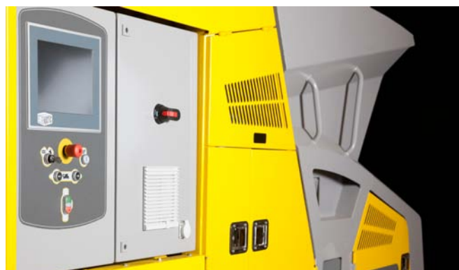
The touch-screen interface enables efficient production control and utilization of history data. Its three access levels prevent uncontrolled entries.
