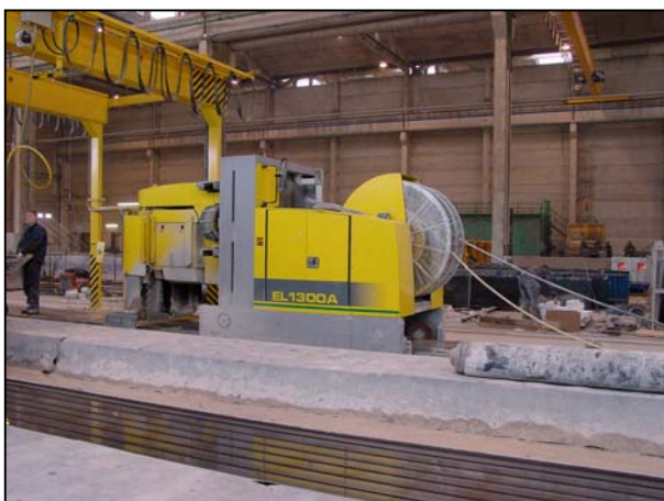
In the ELiPOS module, the product data from ELiPLAN is transferred into cutting information for automatic sawing.
