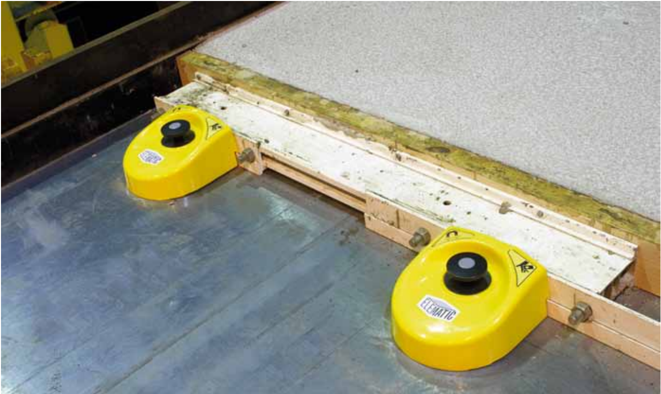
The Elematic Push-Button magnets holds strongly throughout the casting process
