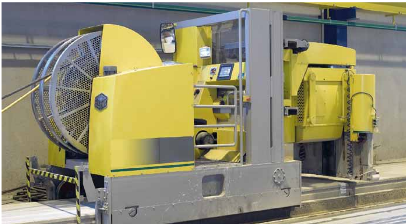
Elematic offers automated EL 1300 saws for cutting elements up to 520 mm.
