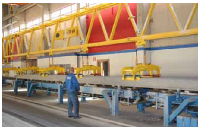
CutMaster lifting a 40 m long hollow-core slab.
